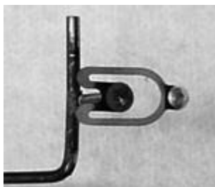
This main tank transmitter didn't survive due to the extensive corrosion.
