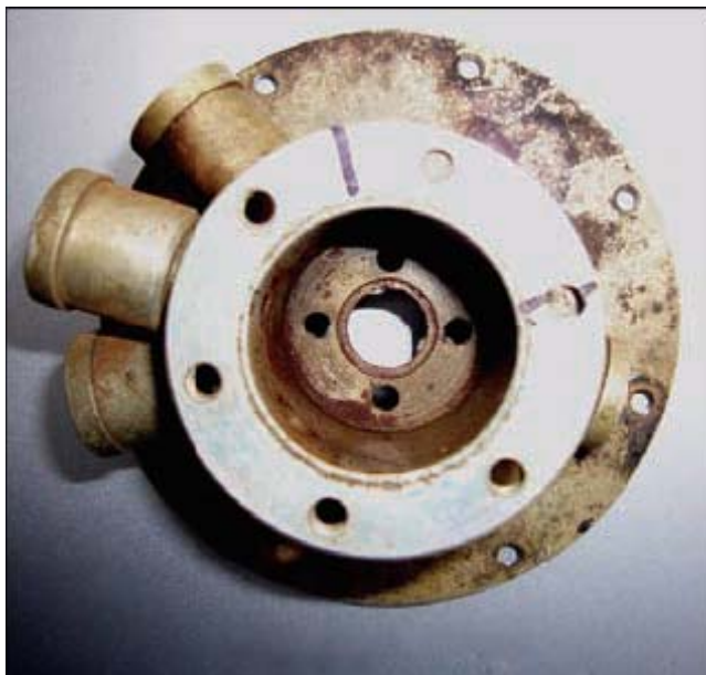
Corroded fuel selector body
