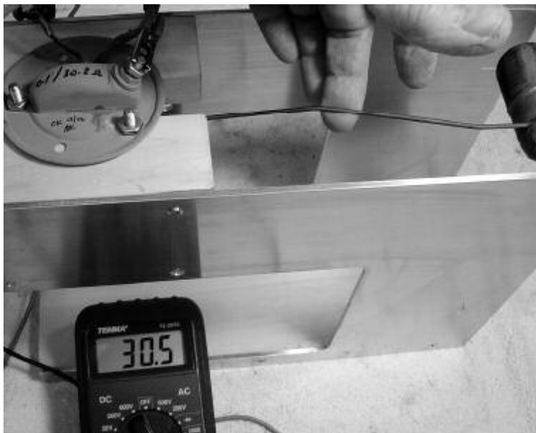
A full-range test must be 29.6 to 31.3 ohms for all except the Comanche 400 auxiliary transmitters (they require two transmitters).
