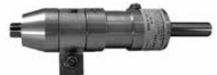
STC SHIMMY DAMPER KIT ALH-001 & ALH-002 APPROVED FOR PIPER MODELS PA24, 30, & 39 SER.
