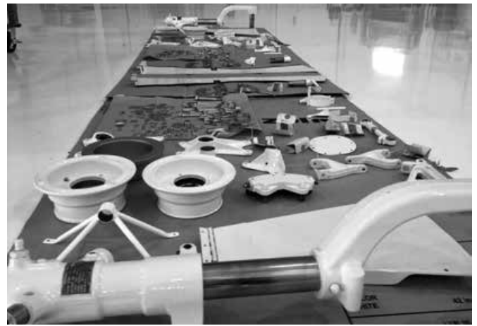
All main gear parts back from refinishing (steel and aluminum).
