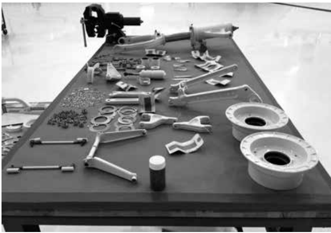
All nose gear parts back from refinishing (steel and aluminum).
